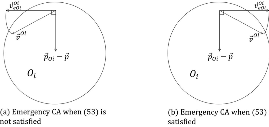
Fig. 13. Emergency CA: USV is already in the hazardous area of O_i . The circle represents the expanded obstacle.
