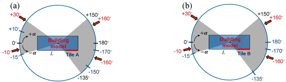
Fig. 4. Wind directions used in training (indicated by red arrows) and testing set (indicated by blue fonts) of SRCNN model for (a) Tile A and (b) Tile B. The wind direction range concerned in PoliMi test is represented by the grey zone.
